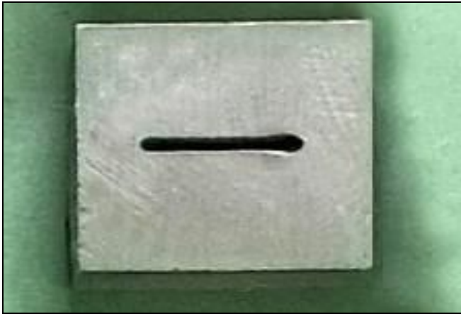
Figure 1 Photograph of specimen cut using AWJ
