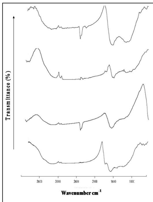
**Figure 1 – FTIR spectrum of activated carbon fiber**
