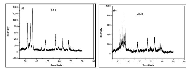
Fig1: XRD pattern of nano ZnO obtained from Zn(CH<sub>3</sub>COO)<sub>2</sub> by Conventional MW irradiation
