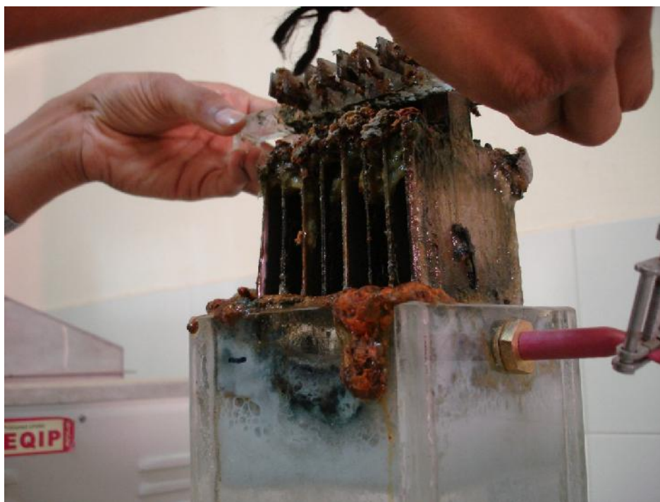
Fig 6. Electrodes just after ECC
