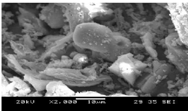
Figure 3: (a) SEM and (b) EDS of bagasse ash
