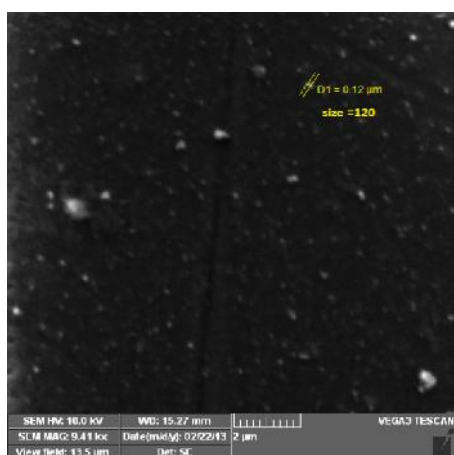
Figure 3: SEM Micrograph of silver nanoparticles formed from OB extract
