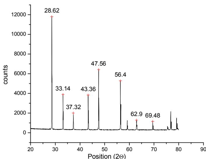
Fig.2 : X-ray diffraction profile of the  $\text{CeNiO}_3$
